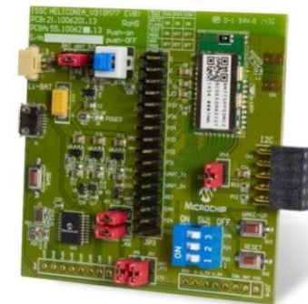
BM77 Bluetooth® 4.0 Dual-Mode Evaluation Board (Part # EV77SPPS3MC2A)
