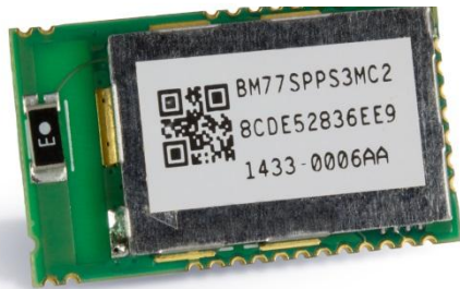
Bluetooth® 4.0 Dual-Mode Shielded Module (Part # BM77SPPS3MC2)
