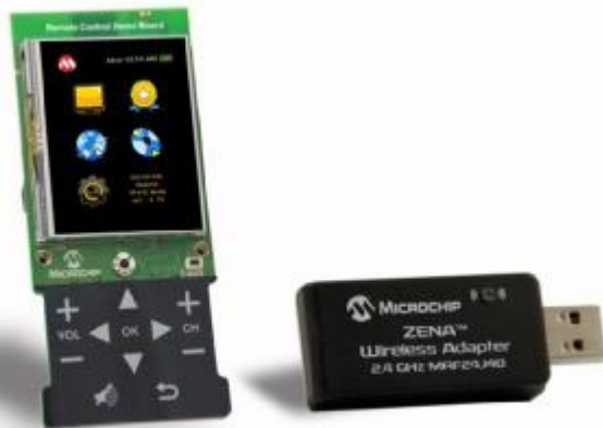
Remote Control Demo Board with ZENA Wireless Adapter (Part # DM240315-2)
