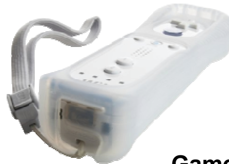
Game Controller: Original version had significant off-drains leading to frequent battery changes
