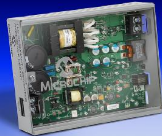
Microchip's DC/DC LLC Converter Reference Design
